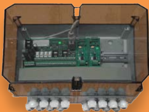
wall box to cover 1x LCM connecting module relays & terminals (if required) WBC 210.1.0.0
